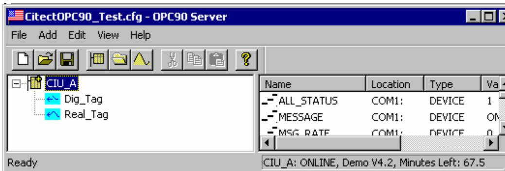
Figure 14 - Create a New OPC90 Server Configuration
