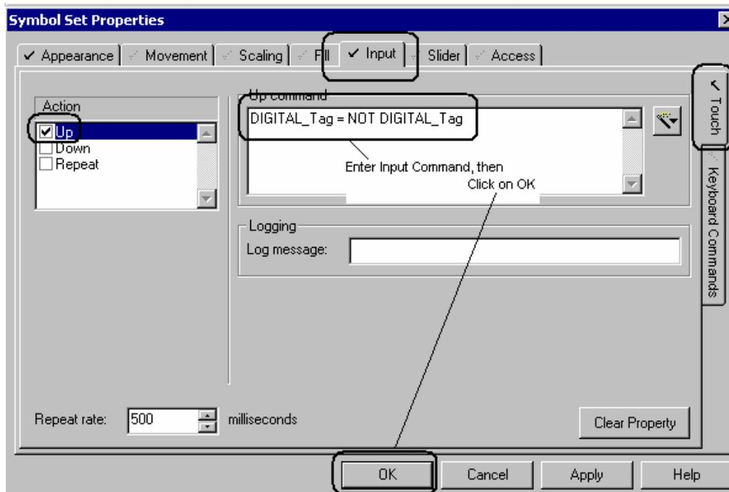
Figure 8 - Configure the Digital Symbol to Toggle on Mouse Click
