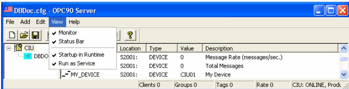
The last step is to configure the MUXCIU block, (called DBDOC in our example) to select a PC COM port that will be used to communicate with the DBDOC CIUMON program. This port will respond to CIUMON as if it were the actual ABB Bailey CIU. Right click on the OPC90 block named DBDOC and select properties to see the following dialog:
