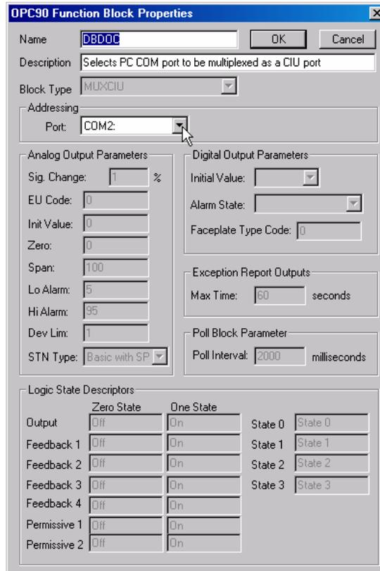
As can be seen by this dialog, the block name is DBDOC and it is of the type MUXCIU which is associated with PC COM2 port. Unless there is a specific reason to utilize a different PC COM port this setup can be left as is. Select the Edit->Ports menu item and verify COM2 is set for 115200 baud. The dialog should appear as:
