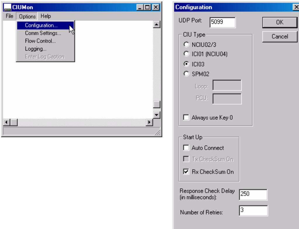
Fill in the UDP port (consult DBDOC documentation) and select the CIU type that best fits the type attached to OPC90. If the system is Network 90 the selected type is NCIU02/03. If the system is Infi 90 the selected type is ICI03 (SCSI CIU) or ICI01. Fill in the other fields as shown. Next select Options->Comm Settings.. which will bring up the following dialog:
