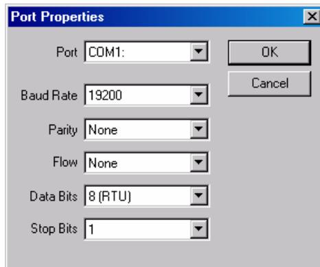
Use this dialog to match the PC COM port settings to the CIU port settings. Generally only the baud rate setting needs to be adjusted.
