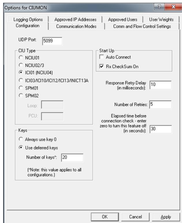
Fill in the UDP port (consult DBDOC documentation) and select the CIU type that best fits the type attached to OPC90. If the system is Network 90 the selected type is NCIU02/03. If the system is Infi 90 the selected type is ICI03 (SCSI CIU) or ICI01. Fill in the other fields as shown. Next select Options->Communication Modes which will bring up the following dialog:
