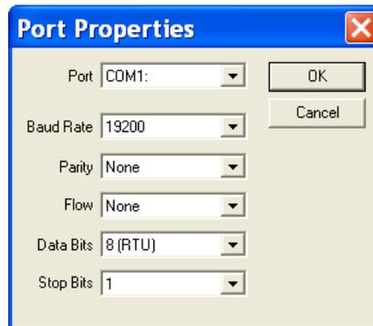
Use this dialog to match the PC COM port settings to the CIU port settings. Generally only the baud rate setting needs to be adjusted.
