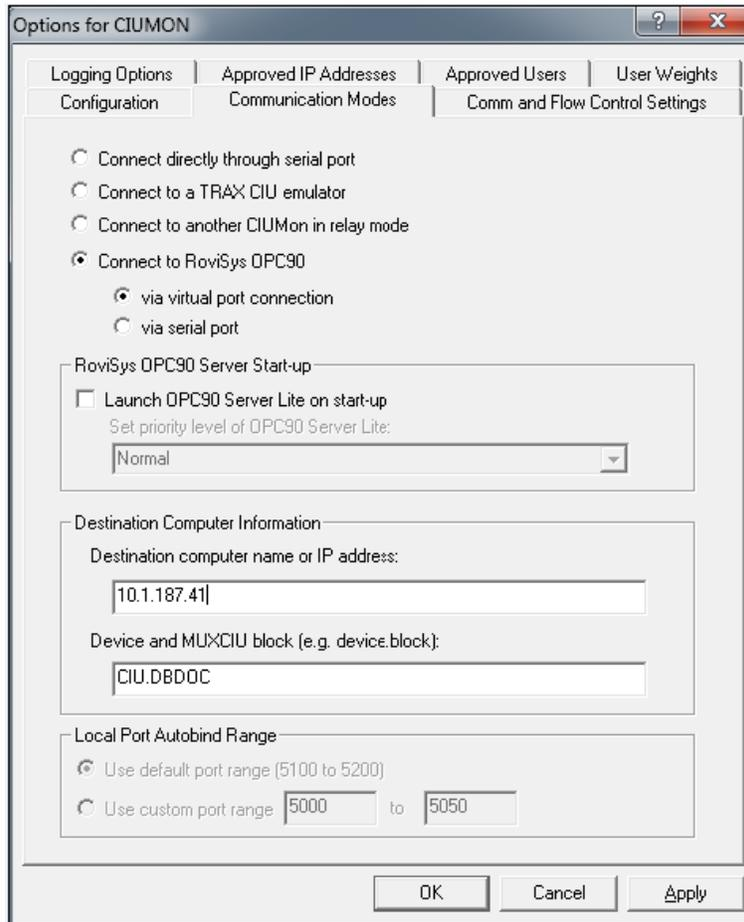
Select Connect to RoviSys OPC90 via virtual port connection, fill in the IP address or computer name of the PC running OPC90 and the name of the OPC90 Device block and MUXCIU block (CU.DBDOC in our example). Set the data characteristics shown by this example which concludes setup of CIUMON.
