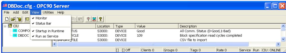
The last step is to configure the MUXCIU block, (called DBDOC in our example) to select a PC COM port that will be used to communicate with the DBDOC CIUMON program and one for COMPOSER. These ports will respond to CIUMON and COMPOSER as if they are the actual ABB Bailey CIU. Right click on the OPC90 block named DBDOC and select properties to see the following dialog:
