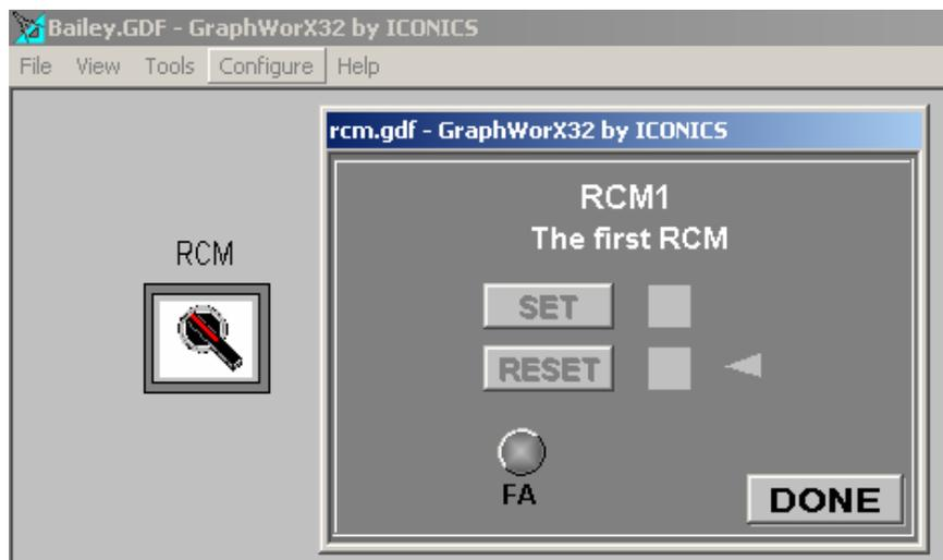
Below shows the configuration of the RCM symbol for use with the faceplate. To configure this faceplate the user must configure these three parameters in the switch symbol. By double-clicking on the switch symbol you will call up the
