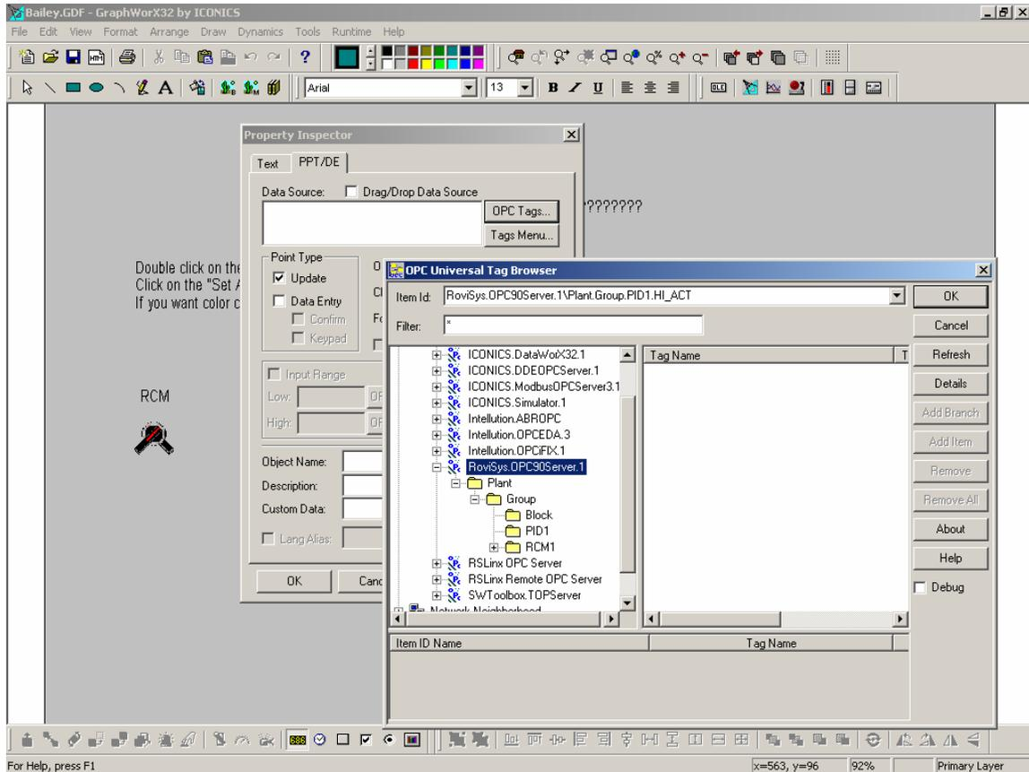
The following example shows the setup of an example with the OPC Server "Device" = "Plant" and the "Group" = "Group". By using the browse feature in the Iconics and selecting the Data Access to "RoviSys.OPC90Server.1" you will find all the tags you created in the OPC server.
