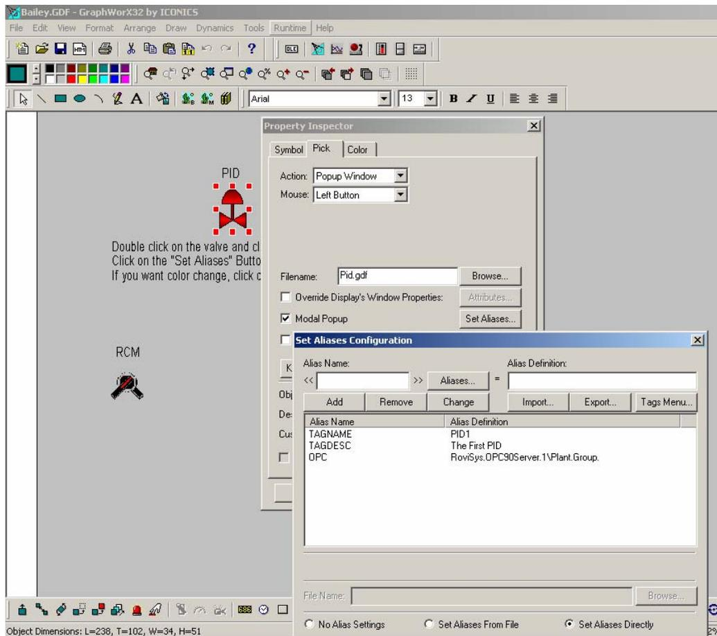
Below is the picture of a switch with the RCM faceplate associated with it. By clicking on the switch in runtime the operator can call up this faceplate.
