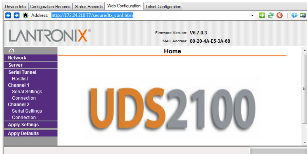
Click on "Network" to setup a fixed IP address for the UDS 2100. It will display the following information. Pick an IP address that is consistent with the network. Obtaining an IP address via DHCP is not recommended. It could change over time which would prevent OPC90 from accessing the device. Enter the data and click the OK button.
