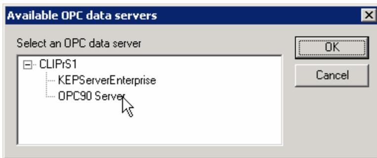
Click ok to accept. Or to setup redundant OPC90 servers, select the Redundancy tab in the OPC Data Server Properties dialogue, otherwise click ok and skip past the next step.
