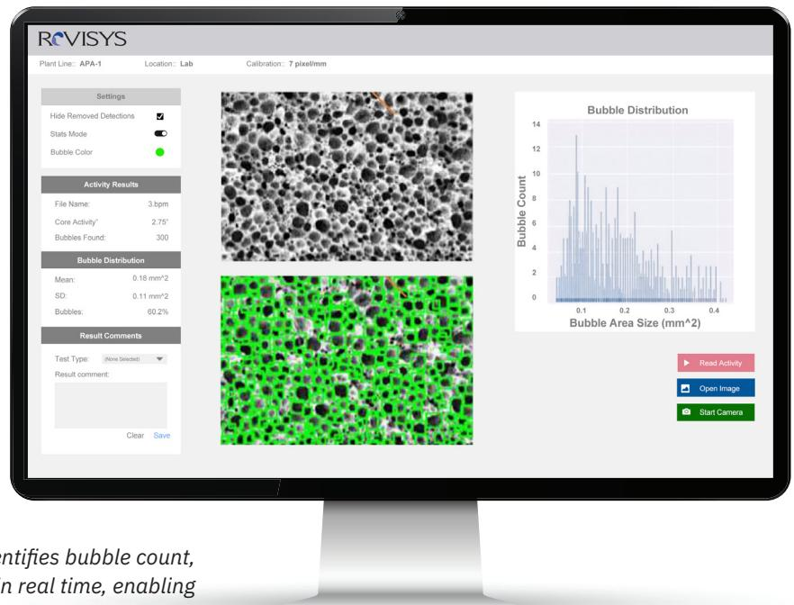
*Computer vision analysis identifies bubble count, size, and density patterns in real time, enabling instant quality grade prediction.*
