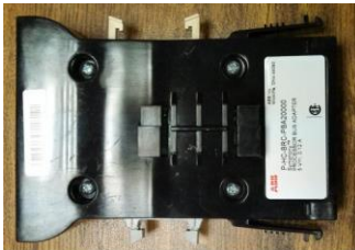
Process Bus Adapter (PBA)
